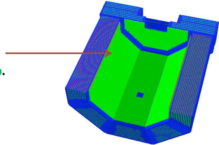
Layout of PANDA muon system (barrel&endcap) without yoke
