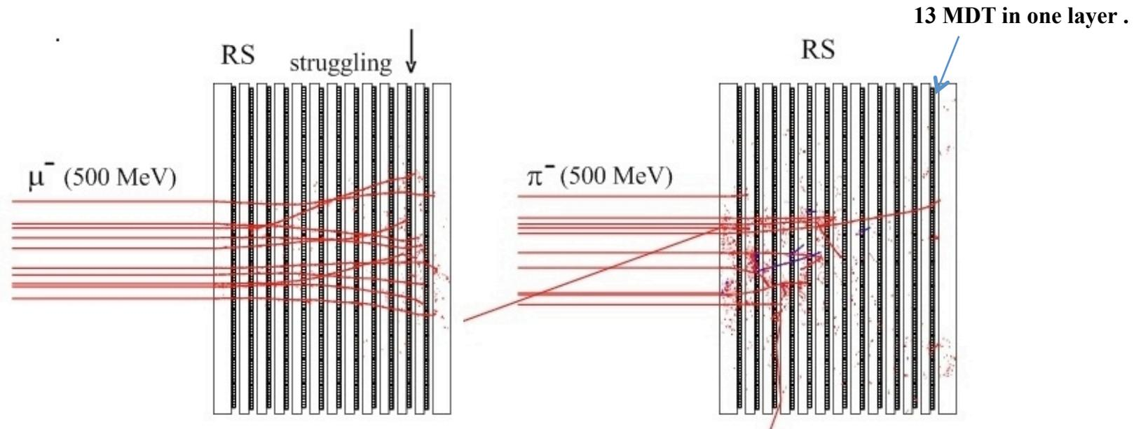
Response of RS to muons and pions at kinetic energy of 500 MeV.
