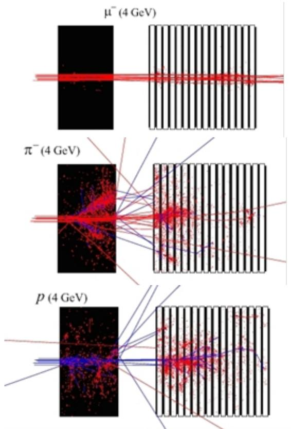
At high energies hadron mostly produces a hadronic shower whereas a muon has a sample of “straight” line spoiled by the multiple scattering. This situation is true for the Forward Spectrometer where particles enter with relatively high energies.
