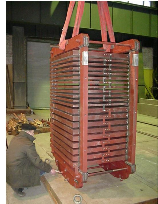
The dynamical energy range depends only from the number of layers of sampling calorimeter. We come to the most important future of RS: the muons can be distinguished from hadrons by the range in sampling calorimeter.
