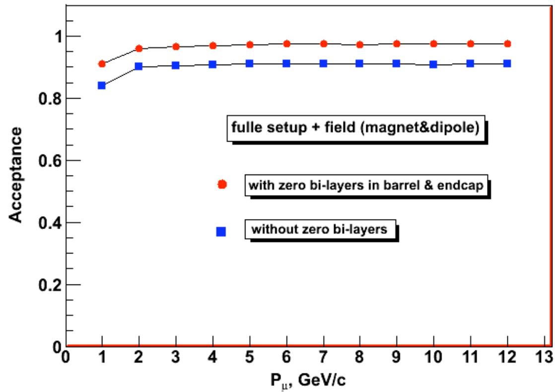
The calculated efficiencies are: 91% (at 1GeV) and 98% with “zero” layers
