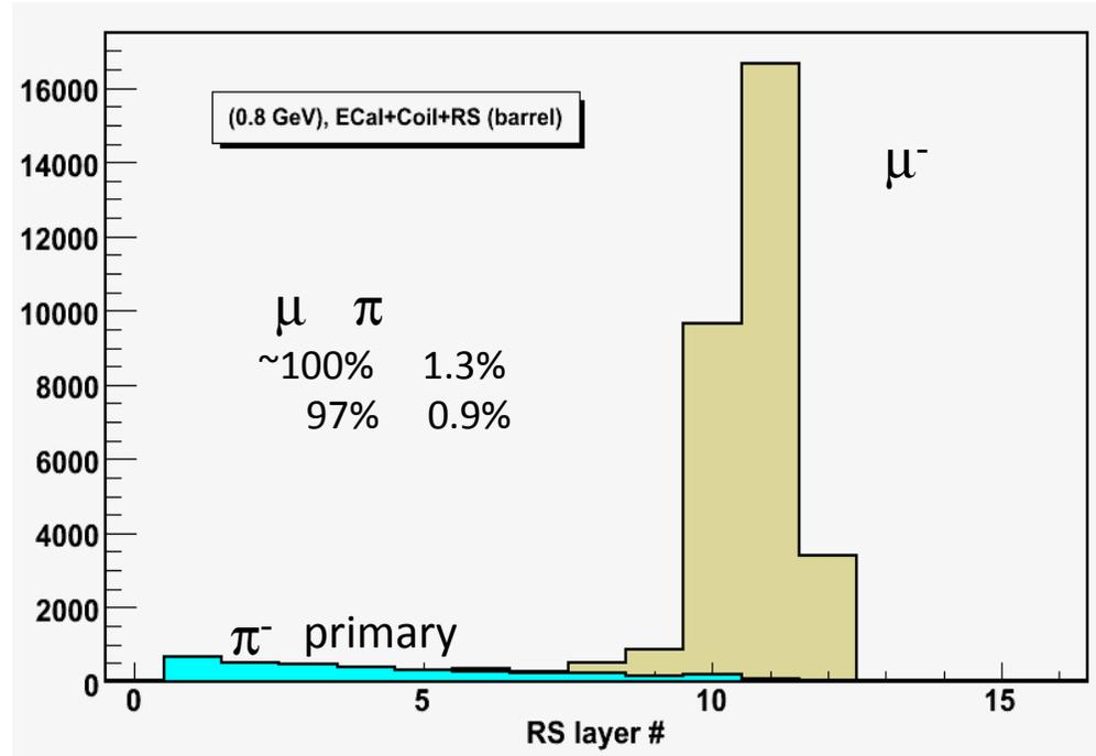
Superposition of distributions of particle ranges in RS for the case of pion and muon beams with initial kinetic energies. Distributions of particle ranges (in number of layers) for muon and pion (dashed) cases at initial beam energies of 800 MeV.
