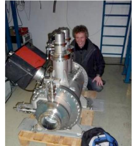
Vacuum tank with slot-coupler (FZJ)
