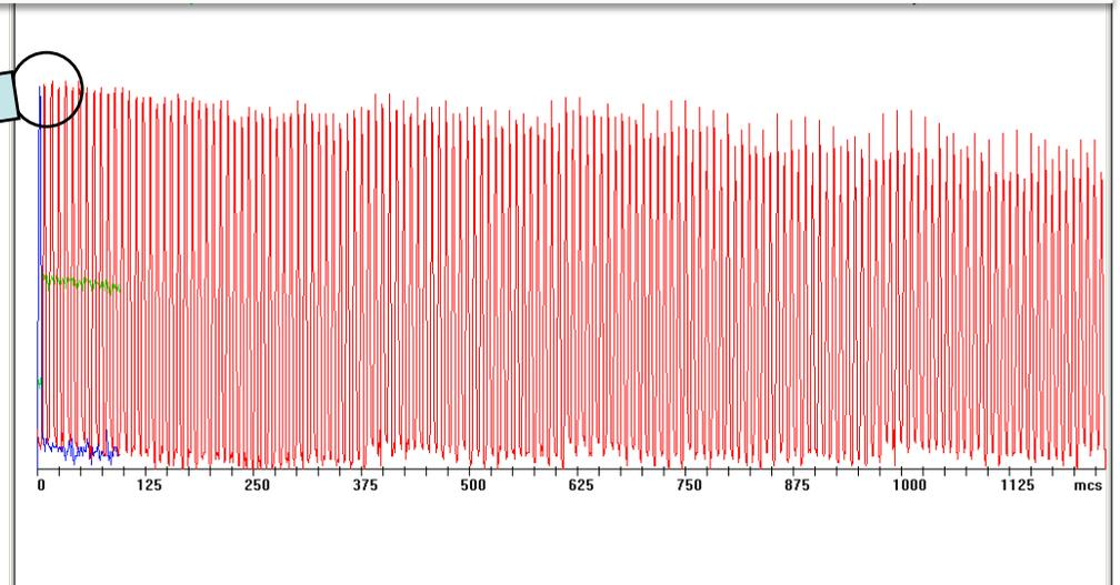
One of the most important results of 42<sup>nd</sup> run: decrease of particle losses at injection. Now 30%, before 70%
