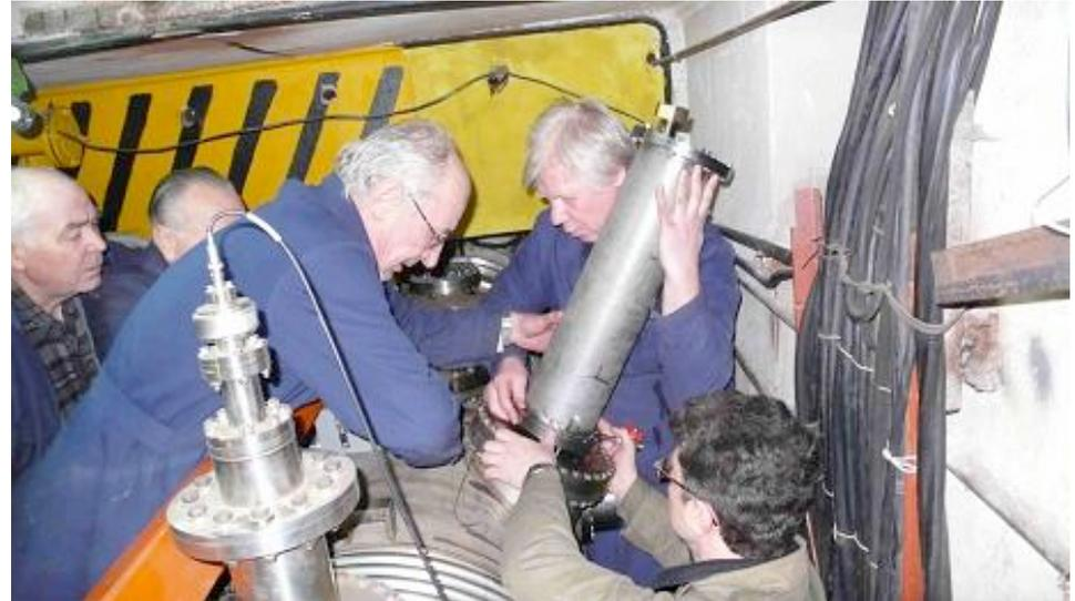
Prototype of new high voltage power supply for the electro-static septum was constructed and successfully tested up to **220 kV** (existing septum power supply allows up to 110 kV only – it corresponds to 2,3 GeV/n extracted beam).
