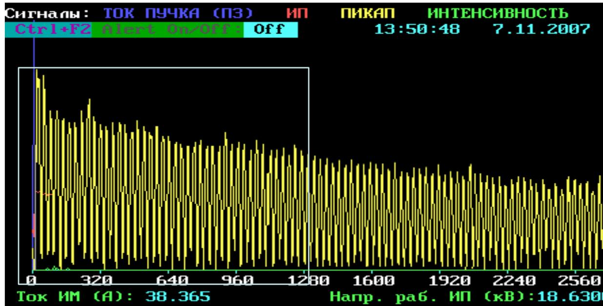
First 6 revolutions (about 50  $\mu$ s) of the deuteron beam in the ring after the orbit correction: Blue line is the injected beam intensity from LU-20, red line: the pick-up signal
