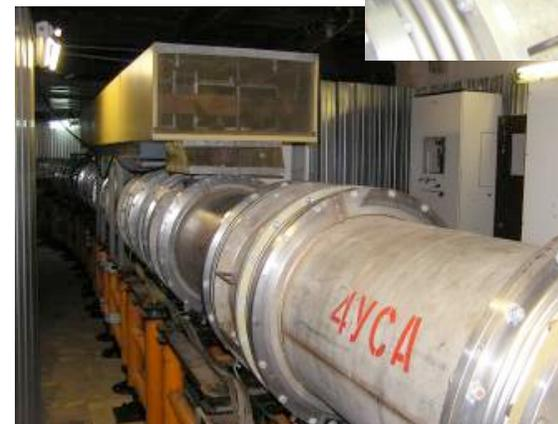
B field from 300 Gs (injection) up to 20000 Gs (max. acc) – factor of 700
