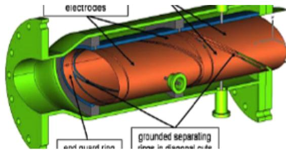
**New (elliptical) pick-up station prototype for Nuclotron (GSI design).**
