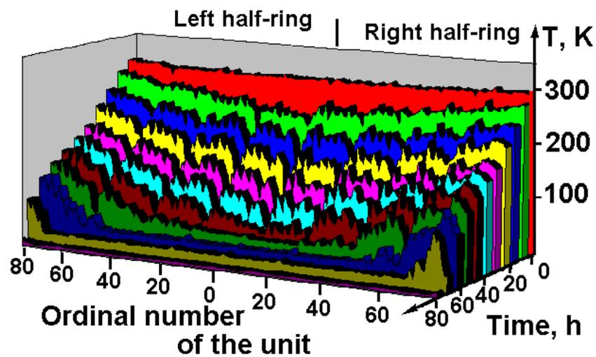
Temperature distribution of the helium cooling gas (30 hours after starting)
