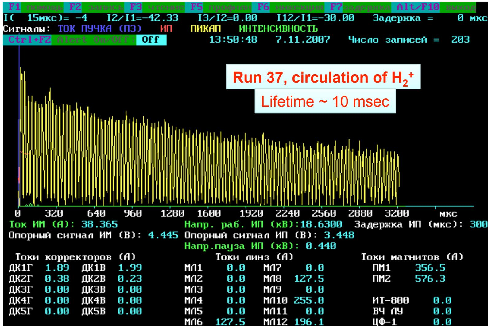
Crosssection decay of  $H_2^+$  ions on Nitrogen at Energy 5 MeV/n ~  $10^{-16}$  cm<sup>2</sup>
