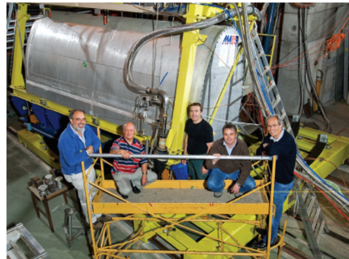
› Liquid Argon Calorimeter The 'accordion' calorimeter is composed of 4000 electrode-absorber layers in ultra pure liquid Argon to maximise stability, granularity and speed.
