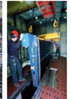
› Tile Calorimeter - Module after module is carefully stacked and surveyed to form a perfect eight-meter tall cylinder, each part placed with millimetre accuracy.
