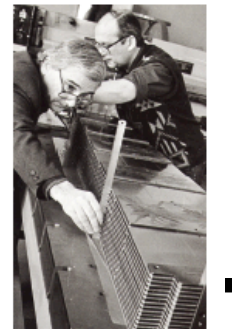
› Tile Calorimeter - Half a million pieces of blue scintillator plastic, 187'000 pieces of green fibre and half a million plates of steel make up the multi-layered tile calorimeter.
