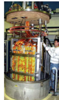
› Liquid Argon Calorimeter The 'accordion' calorimeter is composed of 4000 electrode-absorber layers in ultra pure liquid Argon to maximise stability, granularity and speed.
