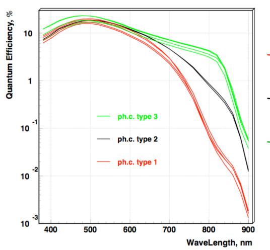
Type 1: Na<sub>2</sub>KSb(Cs) Dark rate ~ 0.5 kcps/cm<sup>2</sup>
