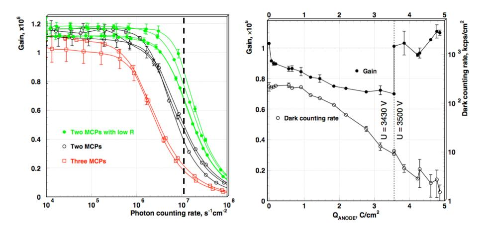
Lifetime measurements at counting rate of  $10^7 \text{ s}^{-1} \text{ cm}^{-2}$ where gain decreases by 20-30%
