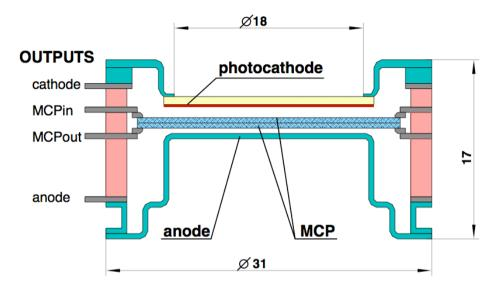
Manufacturer: "Ekran FEP" (Novosibirsk) Borosilicate glass window Multialkali (Sb-Na-K-Cs) photocathode Maximum QE at  $\lambda$ =500nm Two MCPs with channel diameter of 7  $\mu$ m Channel bias angle 13° Single anode
