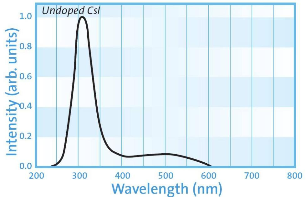
**Figure 1.** Scintillation emission spectrum of CsI(pure)
