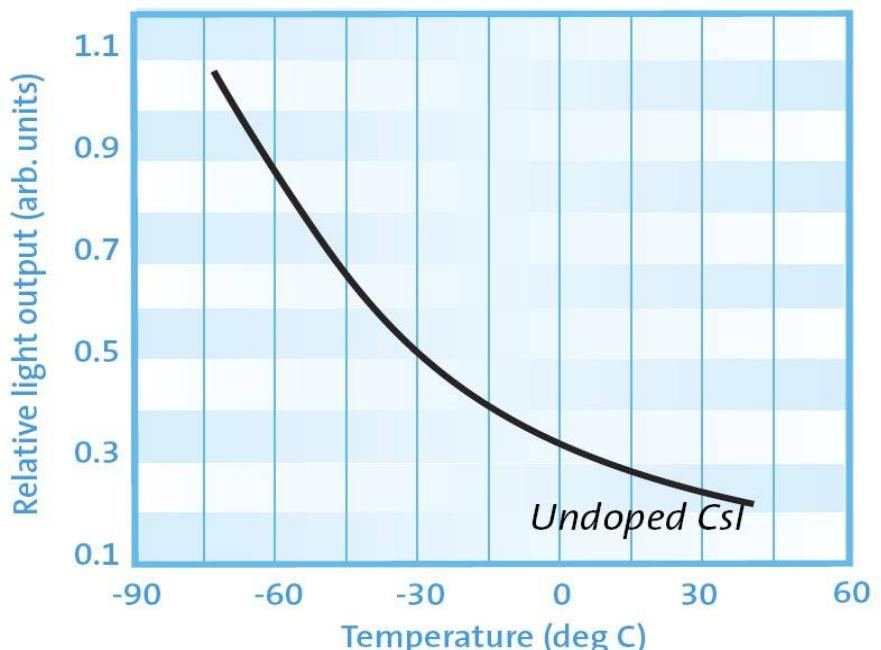
**Figure 2.** Relative light output as a function of temperature for CsI(pure)
